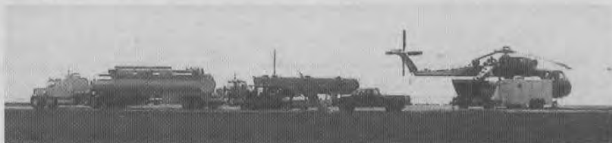
The Erickson Air-Crane helicopters require an entourage of helicopter mechanics, jet fuel trucks and other support vehicles. Their special design allows them to lift 25,000 pounds.
